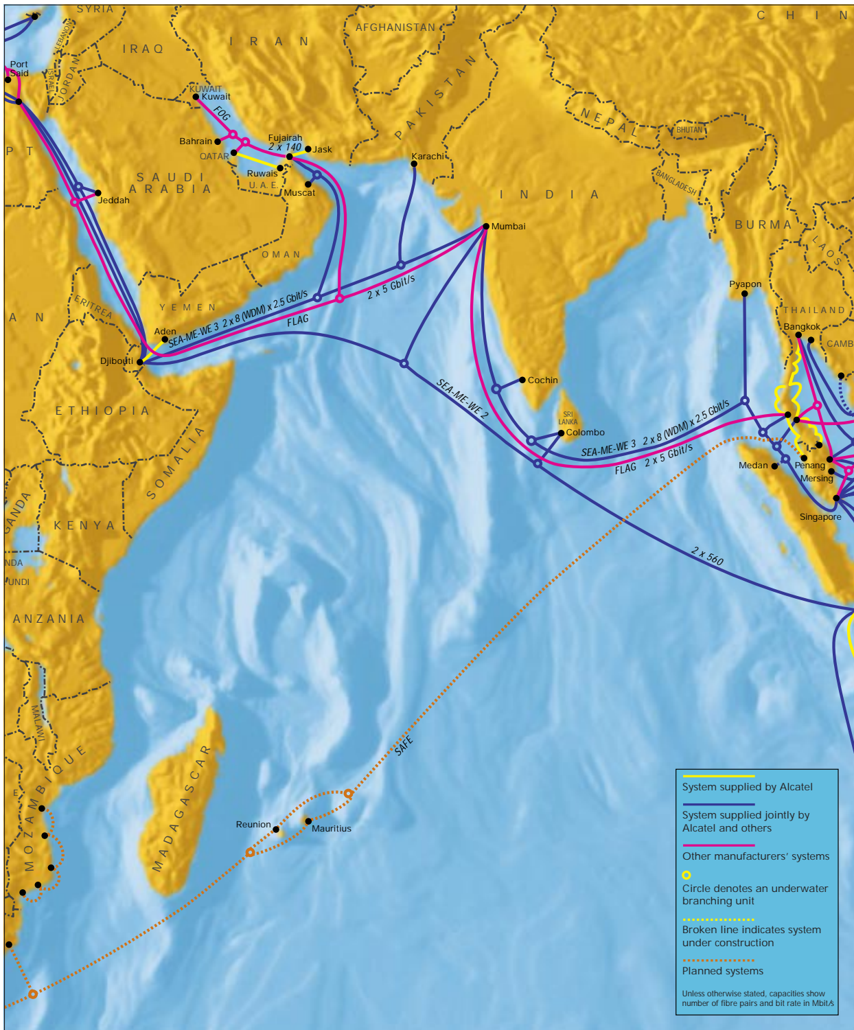
Figure 3.2: Alcatel's Indian Ocean and Middle East optical fiber submarine systems.
