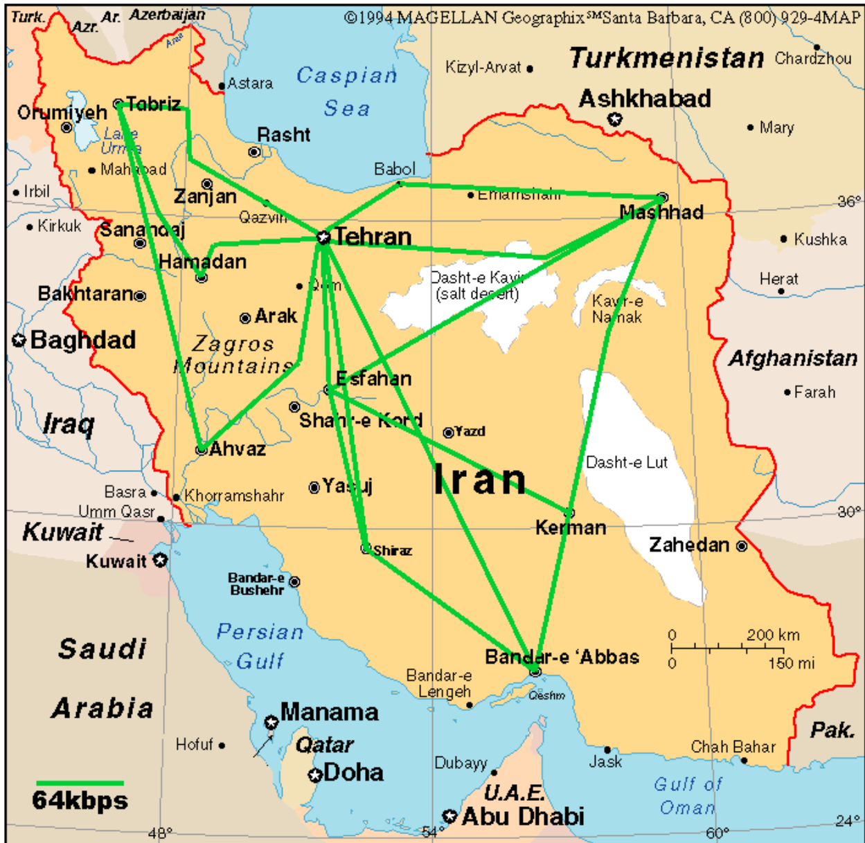
Figure 2.1: Iran's inter-city 64 kbps ISDN lines, as of 1997. The network has since been expanded to include many other cities, including Yazd, Orumieh, Zahedan, Arak, and Rasht.
