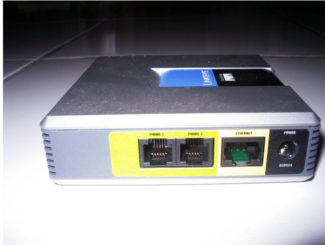
Figure 3.1: With ATA, you can use your PSTN phone for VoIP communication
