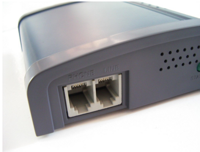
Figure 16.1: ATA Linksys SPA3000 has two RJ-15 sockets on one of its sides
