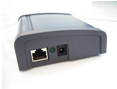
Figure 16.2: ATA Linksys SPA3000 has a RJ-45 socket, power socket and LED indicator on the other side
