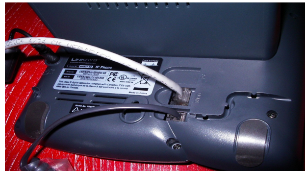
Figure 3.6: IP Phone typically has two RJ-45 ports
