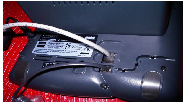
Figure 3.6: IP Phone typically has two RJ-45 ports
