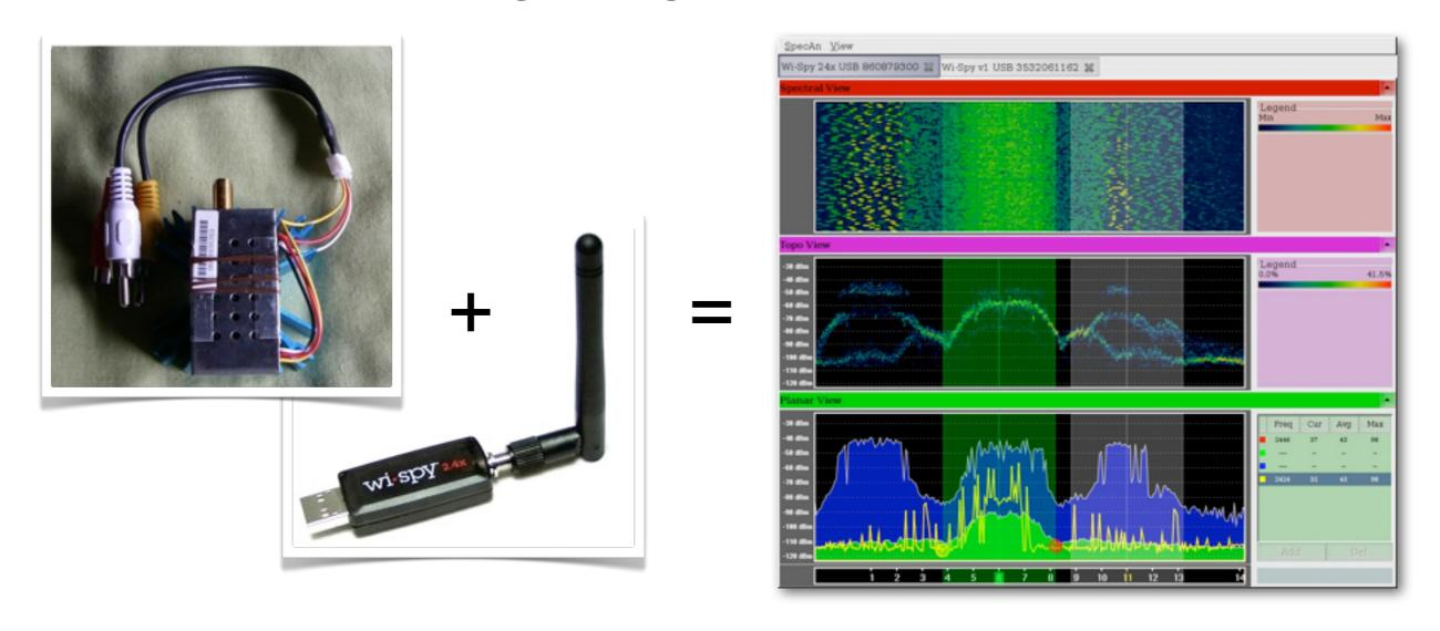
The ideal antenna alignment toolkit consists of a **signal generator** and a **spectrum analyzer**, preferably one of each at both ends of the link.
