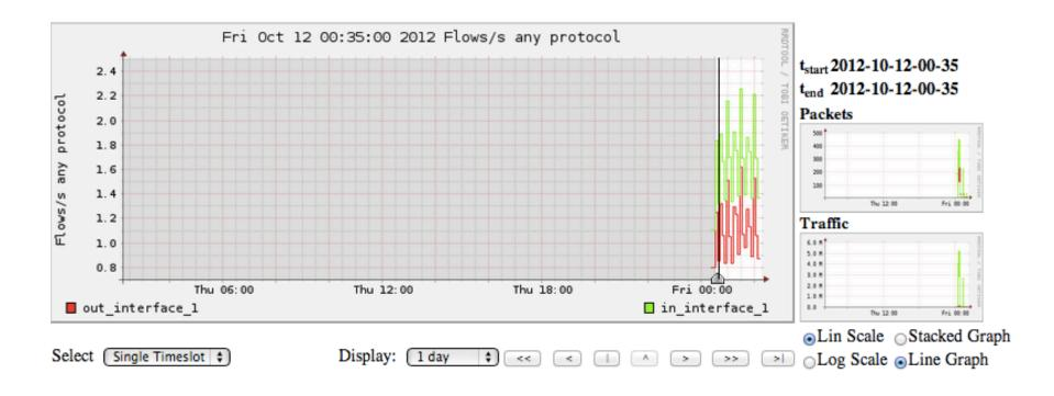
This is a graph of the total traffic passing through the router rtrX on interface FastEthernet 0/0.
