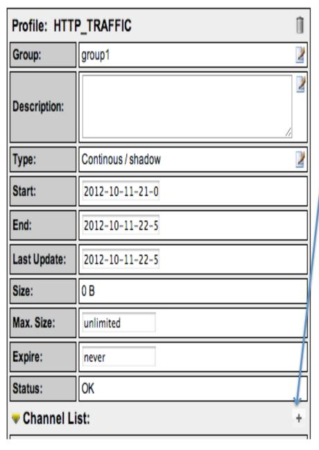
Click on the plus (+) sign next to 'Channel List' at the bottom of the page then fill the next page as below and click on 'Add Channel' at the bottom.
