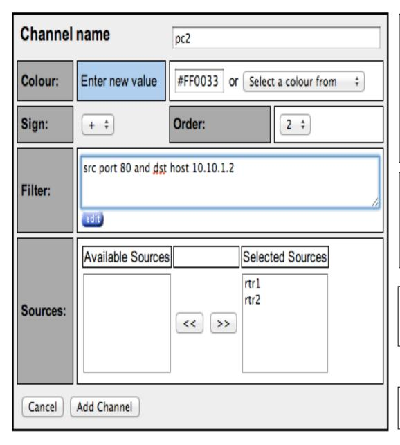
Add another channel by clicking the plus sign as before next to 'Channel List'. Fill the details as shown on the left. Replace pc2 with a pc number that is **NOT receiving flows in your group!** Also, replace the IP address in the Filter to match the IP of the PC in question.
