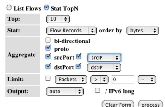
Select the options as on the left. This means, select the Top 10 Flows, Order them by bytes from the highest to the lowest and display information of the source and destination ports and IPs. Then select 'Process'. Analyze the output you get which will look like the below screen.
