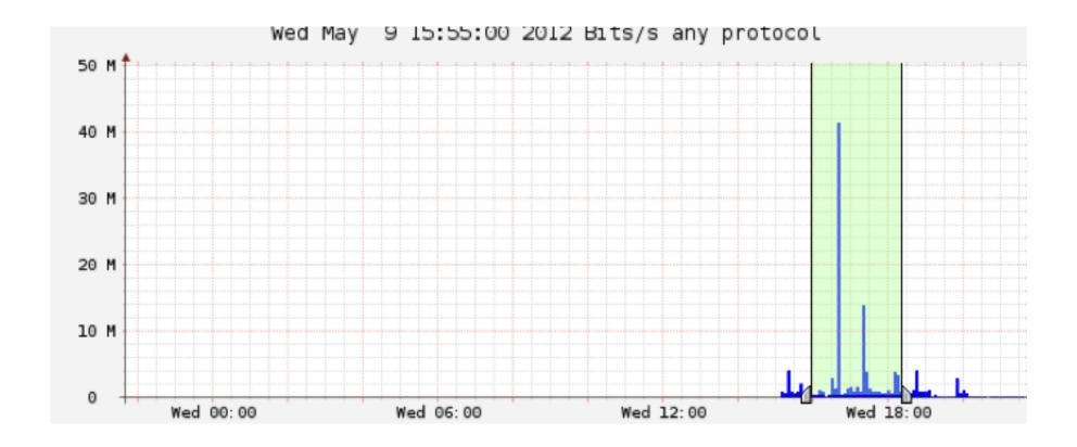
Go to Profile, select the group you created then select 'HTTP\_TRAFFIC'. Then go to the 'Details' tab and select 'Time Window' instead of 'Time Slot' beneath the graph. Choose a part of the graph with activity as above.
