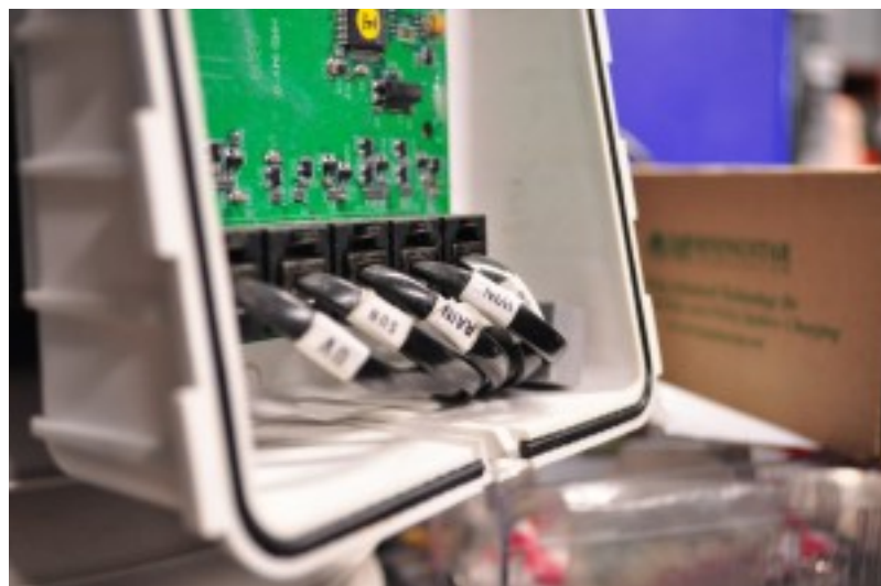
Installation of ASTI Water level Monitoring Apparatus
