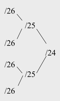
Inversely, if two networks can be "joined" together under the same netmask, which encompasses both networks, then we are *supernetting*.
