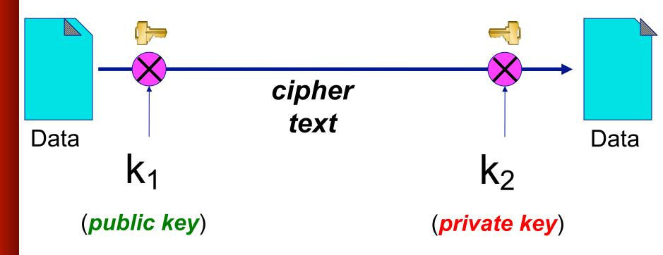
One key is used to encrypt the information, a different key is used to decrypt it.
