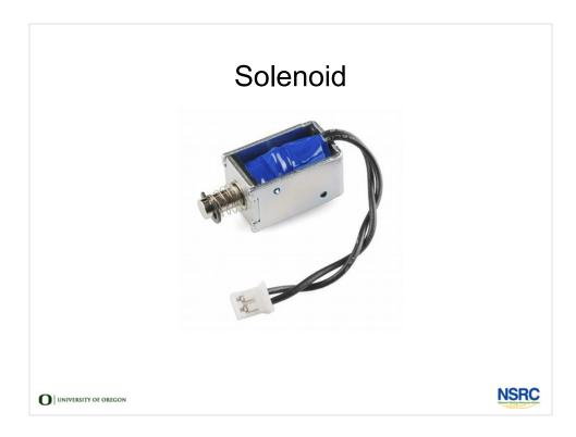
This solenoid is a specially designed electromagnet. The piston in the middle is normally in the out position. When current flows through the solenoid, the piston pulls in. This action could open a valve, activate a mechanical switch, ring a bell, or do anything you could think of.
