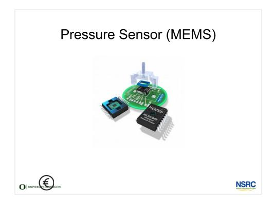
Micro Electrical Mechanical Pressure Sensor - a little machine made of silicon for very precisely measuring pressure.
