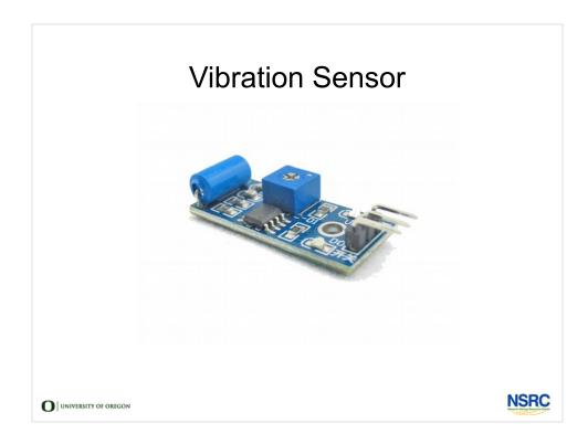
Some vibration sensors are based on piezoelectric devices, and generate voltage in response to being vibrated. Any movement can activate a sensor, the signal from which could be used to wake up a microprocessor and other sensors or actuators.
