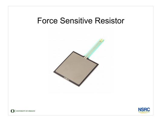
As you press on the surface of a force sensitive resistor, resistance through the circuit goes down.
