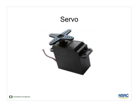
This servo takes DC power and a digital signal from a computer like an Arduino. Send it directions to turn to an arbitrary position like 274 degrees and it'll do it. Servos like this one are commonly used to steer robots and controlled or autonomous vehicles.
