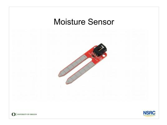
Moisture sensors measure the dielectric constant of soil, or its ability to transmit electricity, and derive an amount of moisture in a particular volume of soil. They can range from inexpensive and inaccurate for a cheap sensor stuck in a pot plant, to expensive and very accurate when properly installed and calibrated to the type of soil they're embedded in.
