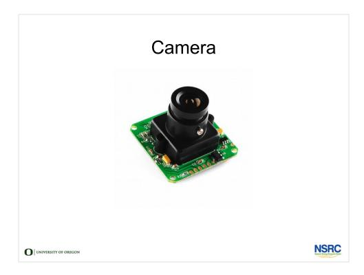
We all know what cameras are good for. I'll just use mine right now. (and now for a selfie). In the world of the Internet of things a camera can do more than just take selfies. Coupled with a Raspberry Pi and some free, open source software called OpenCV, a camera like this can be used for face recognition.
