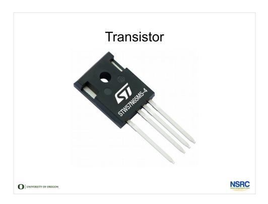
Transistors are used for amplifying or switching electronic signals or power.
