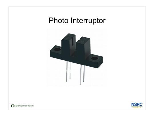
A photo interruptor has a light emitter and a light receiver in-line When something comes between them, a pulse is generated. It can be used to count things or switch things.
