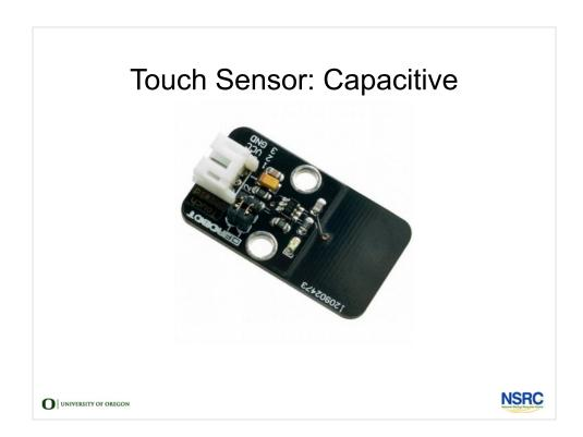
Capacitive Touch Sensors detect when they are touched by a conductive surface, such as a finger.
