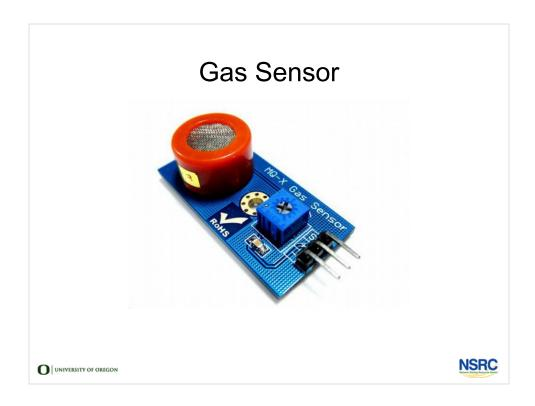
Gas sensors come in a number of different versions, Methane, Butane, LPG, Alcohol, Ethanol, Carbon Monoxide, Hydrogen, Ozone, Benzene, Hydrogen Sulfide, Ammonia... the list goes on. Inexpensive sensors will output a voltage that varies with the concentration of the target gas. As with the formaldehyde sensor, these gas sensors can be important for indoor health and safety in labs, workshops, and manufacturing facilities.
