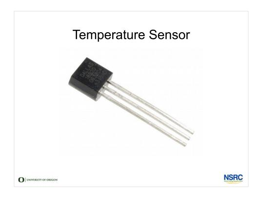
Temperature sensors range in cost an accuracy, but are almost always inexpensive and easy to use. They're so inexpensive, they are often integrated into other sensors and circuit boards. This model uses a 1-wire communications bus, with each device having a 64-bit serial number. Many sensors can be chained together to produce high resolution data.
