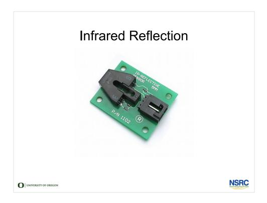
This sensor generates infrared light and measures its reflected strength. One of its applications is to determine distance. Infrared reflection sensing is also used to help robots follow lines, and in optical dust sensors.
