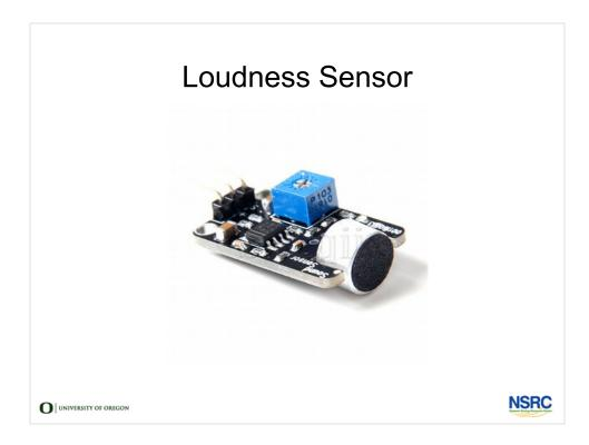
A loudness sensor uses a microphone, an amplifier, and filters to output a digital signal that can be translated into a measurement of the decibel level of sound.
