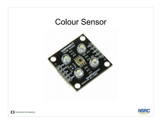
Colour sensors are a bit more interesting to me than cameras. I think this one senses red, green, blue, and brightness, and reports back an intensity You could point one at a machine that has red and green lights, to easily know the state of the machine. You could also use one with a conveyer belt to check or record the ripeness of some fruit or vegetables.
