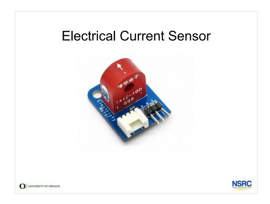
This sensor allows you to pass a wire through it to monitor the current flowing through the wire. You might use it as an electricity meter, or you could use it to keep track of when an automated pump, fan, or light was running.
