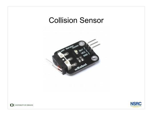
Much of the popularity of small microprocessors like the Arduino is a result of people's fascination with robots. This very rudimentary collision sensor allows a moving device (hopefully moving very slowly) to know when it's hit something else - maybe a wall, another robot, or a shoe.
