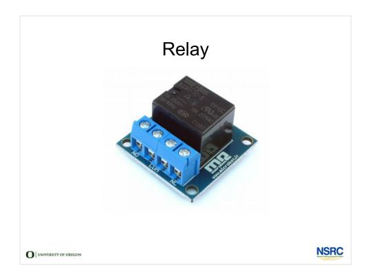
Relays act as a switch for current. This one has three ports: com means common, and is involved in all circuits through the relay. NO means normally open, and NC means normally closed.
