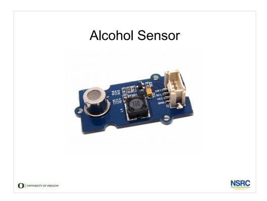
This five-euro sensor can be used to test breath alcohol. It could be used to provide an inexpensive interlock on a machine, a car or a tractor that shouldn't be operated by someone who has been drinking.
