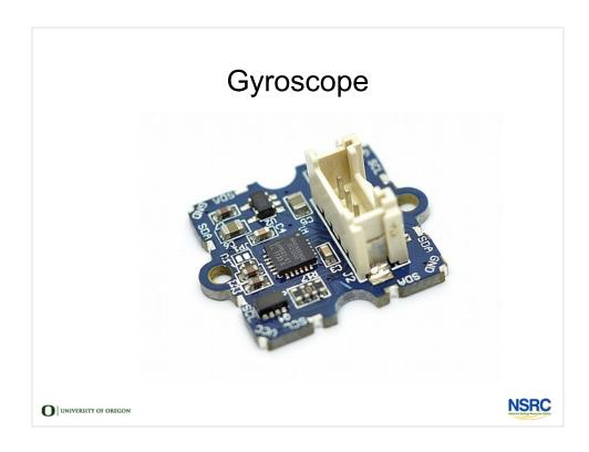
A gyroscope measures orientation in multiple axis.
