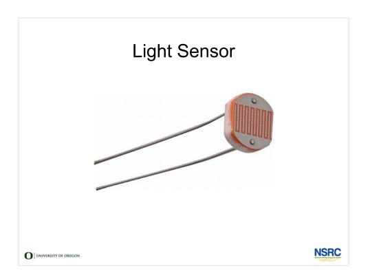
A light sensor, or a light dependent resistor, is a very inexpensive but relatively inaccurate device that will tell you if it's light or dark.
