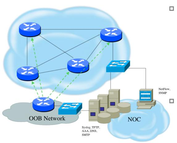
Out-of-band device management should be used to ensure DoS attacks do not hinder getting access to critical infrastructure devices
