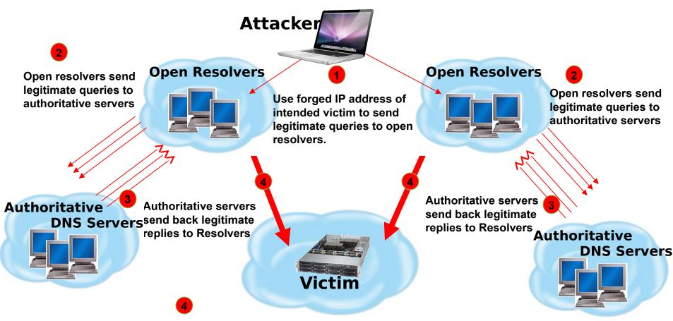
Open resolver legitimate responses create massive DDoS attack to victim's IP address.
