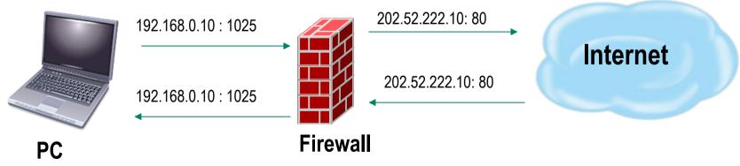
Only allows reply packets for requests made out Blocks other unregistered traffic
