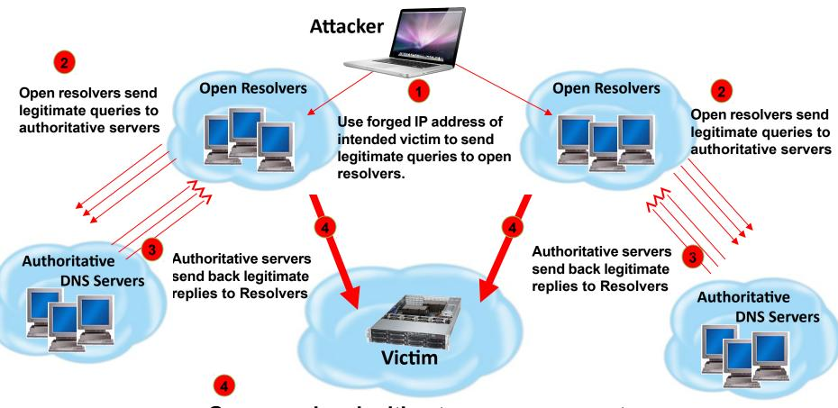
Open resolver legitimate responses create massive DDoS attack to victim's IP address.
