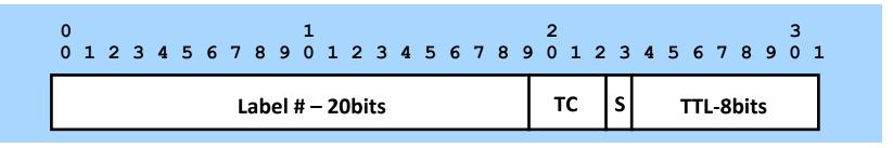
TC = Traffic Class: 3 Bits; S = Bottom of Stack; TTL = Time to Live
