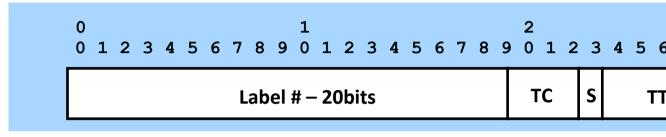
TC = Traffic Class: 3 Bits; S = Bottom of Stack; TTL = Time to Live
