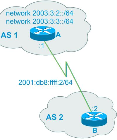
BGP-4 Configurations for IPv6 Link Local Peering
