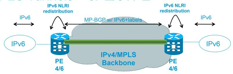
IPv6 packets transported from 6PE to 6PE over Label Switch Path
