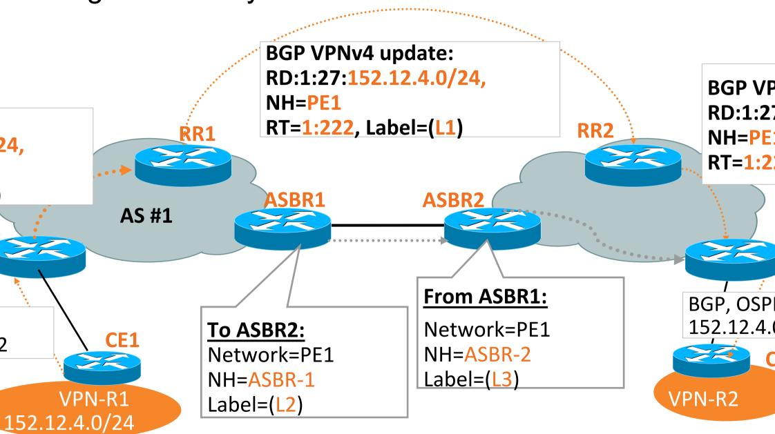
tore PE loopbacks & exchange labels for PE Loopback addresses
