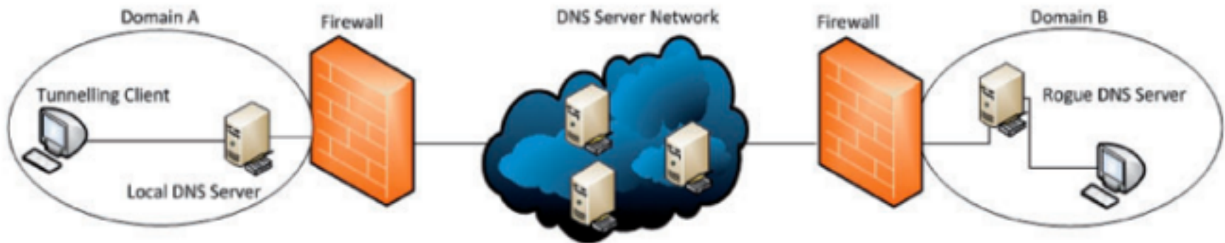
FIG. 1. Entities involved in a DNS Tunnel.
