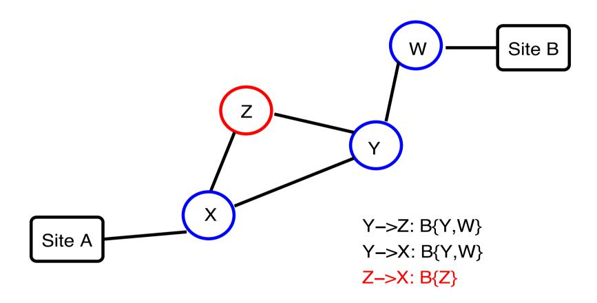
Z claims that it has a shorter path to B than Y does (1 hop versus 2). X believes Z.
