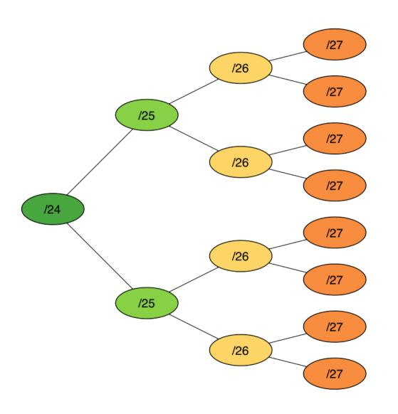
Add one bit to the netmask & the network divides in two This is subnetting
