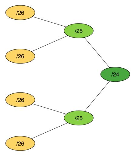
Subtract one bit from netmask & the network joins together This is supernetting
