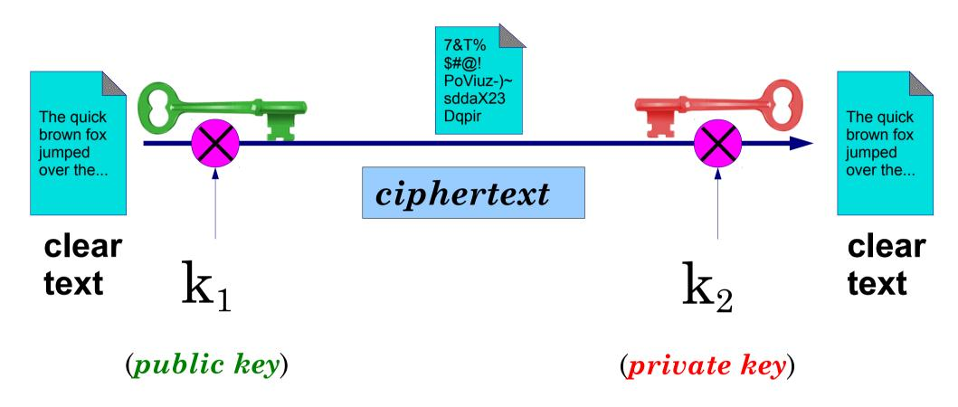
One key is used to encrypt the document, a different key is used to decrypt it.
