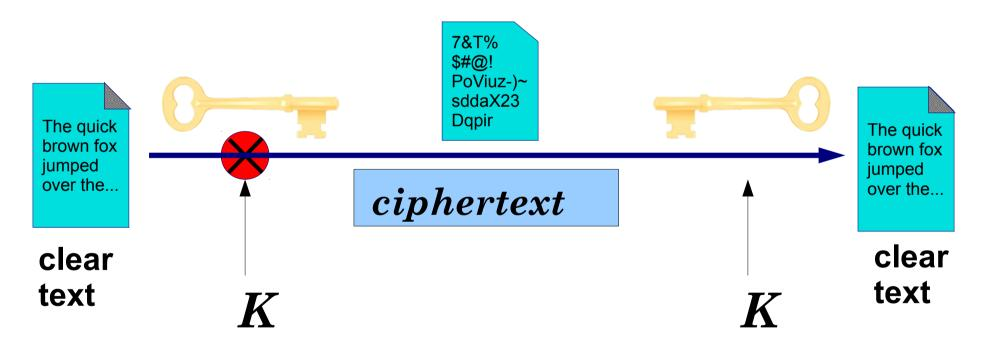
The same key is used to encrypt the document before sending and to decrypt it once it is received
