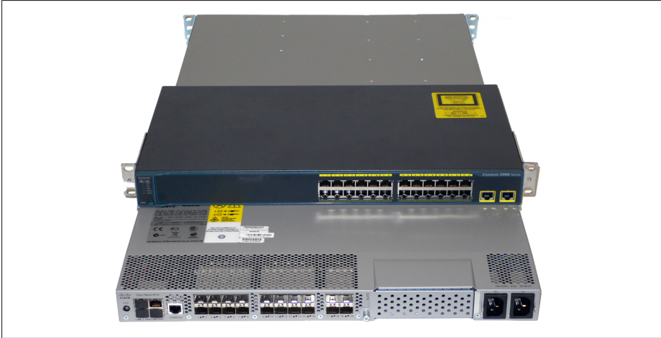
Figure 18-5. Catalyst 2960 on top of a Nexus 5010
