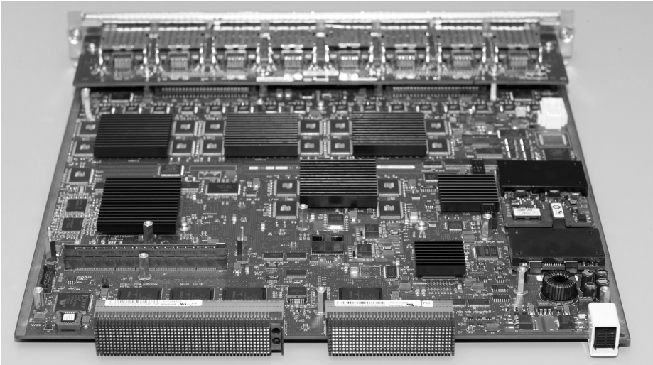
Figure 17-6. Fabric-enabled blade connectors
