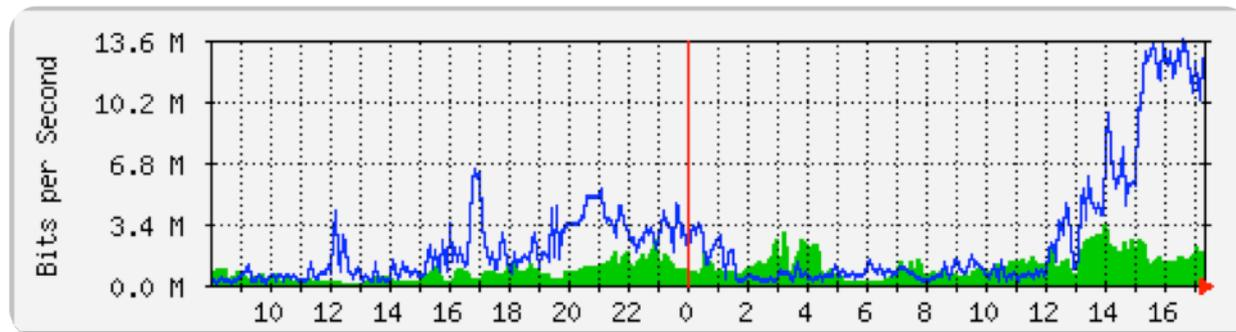
MRTG = "Multi Router Traffic Grapher", grapheur de trafic multirouteur
