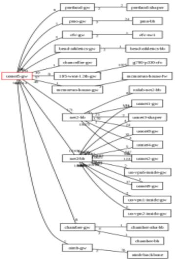
Netdot can dynamically draw the topology of a network or a segment of a network.
